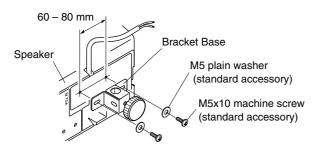
Step 2. Mount the Bracket Stay to the wall or ceiling.
