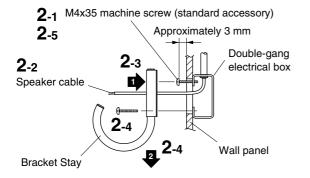
Step 2-1. Temporarily install two of the supplied screws 46 mm apart, and leave them sticking out approximately 3 mm from the wall or ceiling surface. The following figure shows the relationship of the speaker cable outlet hole to the Stay mounting position.
