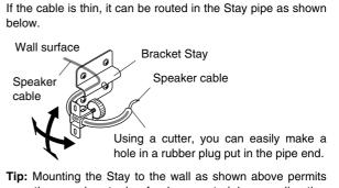
Tip: Mounting the Stay to the wall as shown above permits the speaker to be freely mounted in any direction indicated by the arrows.
